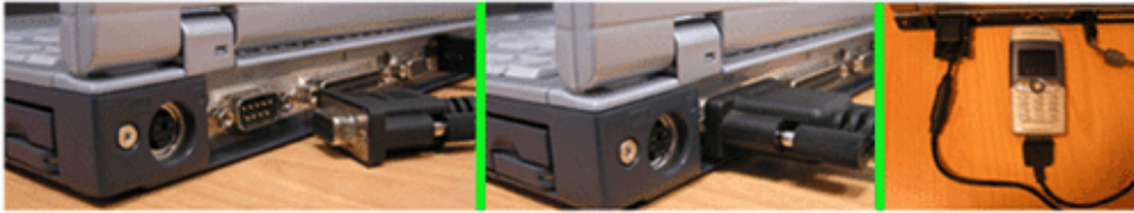
Figure 1 - Attaching the device to the PC with a phone-to-pc data cable
