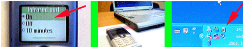
Figure 2 - Attaching the device to the PC with IR connection.
