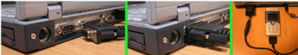
Figure 1 - Attaching the device to the PC with a phone-to-pc data cable.
